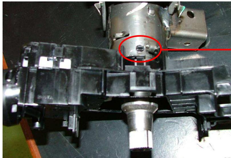
**Insert the light command in the steering column, and be carefull to don't damage the locating in the steering column hole.**
